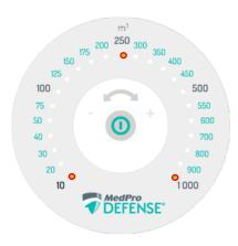
The 10m³ and 1000m³ LEDS flash and the 250m³ LED lights up.
